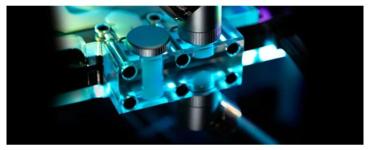
The base of the active backplate is CNC-machined out of nickel-plated electrolytic copper, while its top is CNCmachined out of glass-like cast Acrylic. The rest of the backplate is made of nickel-plated aluminum and it does not come in contact with the liquid. These Vector Active Backplates also feature acrylic terminals that match the top cover. The watertight sealing is ensured by high-quality EPDM O-rings.
