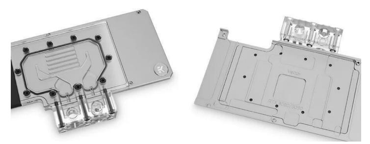
The Vector Active Backplate directly cools the PCB hotspots that are found on the backside of the GPU core and the VRM (voltage regulation module). On the RX 3090, the VRAM located on the backside is cooled, while the RTX 3080 gets cooling for the PCB located around the front-mounted VRAM. Cooling liquid is channeled over all these critical areas.
