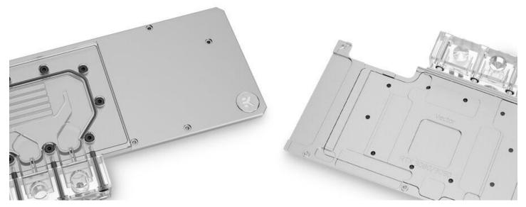
The base of the active backplate is CNC-machined out of nickel-plated electrolytic copper, while its top is CNCmachined out of glass-like cast Acrylic. The rest of the backplate is made of nickel-plated aluminum and it does not come in contact with the liquid. These Vector Active Backplates also feature acrylic terminals that match the top cover. The watertight sealing is ensured by high-quality EPDM O-rings.
