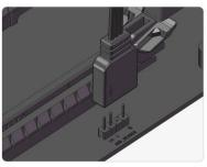
The 5V ARGB adapter cable should be connected to the corresponding motherboard interface in the corresponding direction
