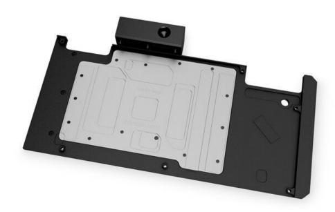
The Vector Active Backplate directly cools the PCB hotspots that are found on the backside of the GPU core and the VRM (voltage regulation module). On the RX 3090, the VRAM located on the backside is cooled, while the RTX 3080 gets cooling for the PCB located around the front-mounted VRAM. Cooling liquid is channeled over all these critical areas.
