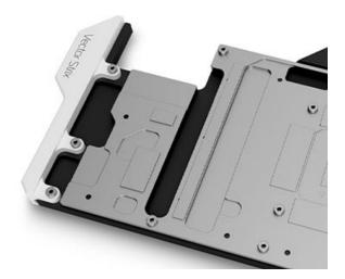
These newly developed water blocks feature optimized flow paths that reduce hydrodynamic instabilities and vortexing (dead spots) inside of them. Additionally, this new design allows the copper cold plate to extend almost the entire length of the PCB, cooling even less important components for maximum efficiency.
