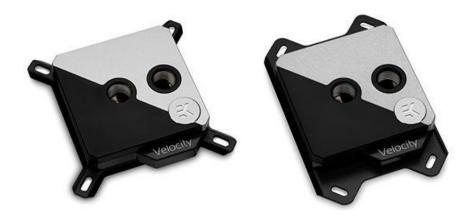
The top is CNC machined out of a solid piece of brass which is nickel-plated black, while the aesthetic cover piece of aluminum anodized in matte black. The purest copper available on the market is used for the EK-Quantum Velocity Strike cold plate which is precisely machined to a dense micro-fin structure. The contact surface itself is machine polished for better contact with the CPU IHS.
