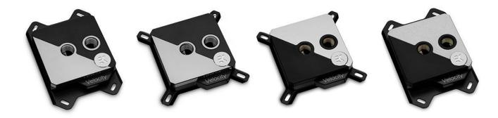
The top is CNC machined out of a solid piece of brass which is nickel-plated black, while the aesthetic cover piece of aluminum anodized in matte black. The purest copper available on the market is used for the EK-Quantum Velocity Strike cold plate which is precisely machined to a dense micro-fin structure. The contact surface itself is machine polished for better contact with the CPU IHS.
