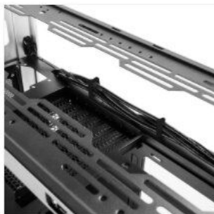
Top fan and radiator mounting holes
