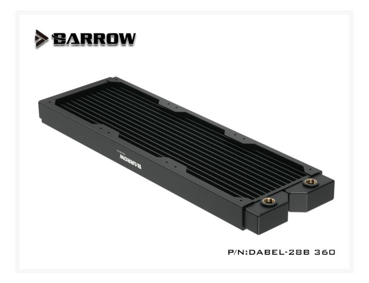
BARROW Dabel-40b series of red copper water cooling standard height of 28MM, suitable for high heat dissipation requirements of standard or large water cooler installation and use. The waterway is made of pure copper material, the brass of the water chamber and the fan mounting bracket are made of stainless steel.
