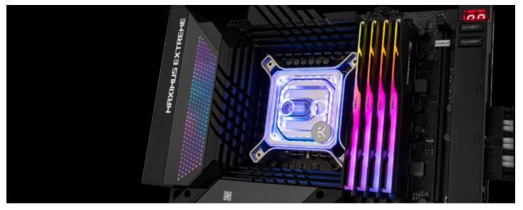
A CNC machined solid brass insert made it possible to significantly enlarge and optimize the cooling engine. Compared to previous generations of water blocks, the fin array has a 50% bigger surface area, all contained in a smaller footprint to ensure maximum compatibility even with mITX motherboards. The copper cold plate uses 0.40mm wide microchannels and 0.26mm thick microfins to maximize the thermal transfer with minimal flow restriction.
