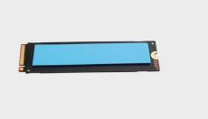
$2. Paste thermal\, grease\, to\, one\, side\, of\, the\, hard\, disk$
