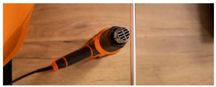
The heat gun is equipped with a digital display, with colored temperature increments, and two buttons for fine adjustment of the air temperature. The air temperature can be adjusted in 30°C increments for the low power setting, and 55°C for the high-power setting.
