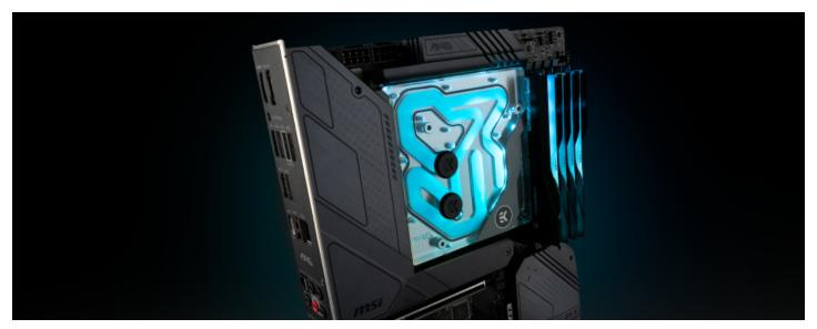
EK® series LiteBlocks utilize the new Velocity² water block cooling engine. This water block directly cools the Intel® 1700 socket-type CPU, as well as the heatsink of the power regulation (MOSFET) module. The monoblock replaces the stock heatsink with a special one that connects to the LiteBlock. They are connected via thermal pads in between them and LiteBlock effectively dissipates heat from the heatsink instead of the VRM directly.
