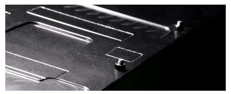
The backplate improves the overall aesthetics of your graphics cards and also provides additional passive cooling for the GPU core, and backside of the printed circuit board VRM section.
