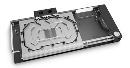
Great care was taken to achieve a symmetrical flow domain by utilizing an internal bridge to secondary components. This was done to ensure the cooling of secondary components without sacrificing flow distribution over the GPU core.
