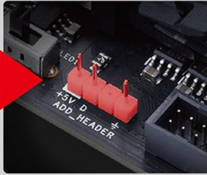
1-2 Connect 4pin ADD RGB header to Motherboard with +5V ADD RGB header.
