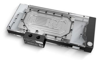
Great care was taken to achieve a symmetrical flow domain by utilizing an internal bridge to secondary components. This was done to ensure the cooling of secondary components without sacrificing flow distribution over the GPU core.
