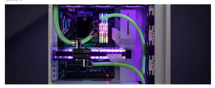
High resistance to leaching was one of the paramount focuses while making this tubing. EK-Loop Soft Tube uses a non-Phthalate plasticizer. It is resistant to degradation and discoloration from Beta, UV, and Gamma rays. All components used in manufacture are US FDA sanctioned for food applications and meet USP Class VI for use in the medical industry.
