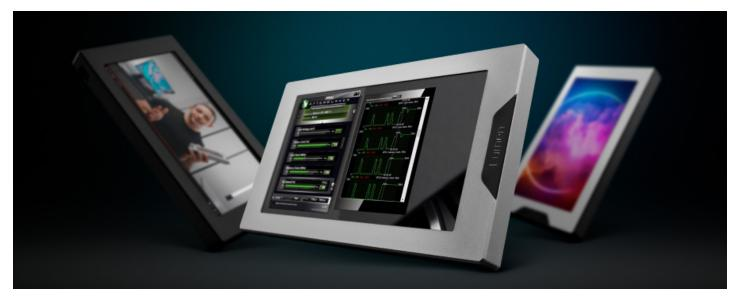
The sturdy anodized silver aluminum frame offers three mounting positions with hole spacing aligned with 120mm fans. This allows the screen to be moved up and down or centered, depending on your preference, while ensuring a high degree of compatibility with most modern cases. This 7" monitor can also be mounted on EK-Loop Angled Bracket 120mm to allow 90-degree rotation and additional positioning options.
