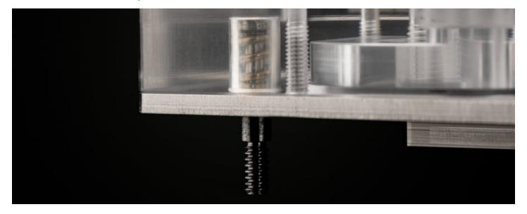
The integrated mounting screws are engineered with a hard-stop design, so once screws reach the end of the thread, the block is perfectly mounted and tensioned. This removes the risks of over-torquing the water block and potentially damaging your motherboard and/or CPU.
