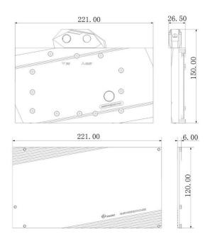
This full coverage block directly cools the video cards core (GPU), graphics memory (RAM), and voltage regulator modules (VRM). By directly cooling these components you can achieve great temperatures along with the ability to reach higher overclocks or extend the overall lifespan of your card by running at below factory temps.
