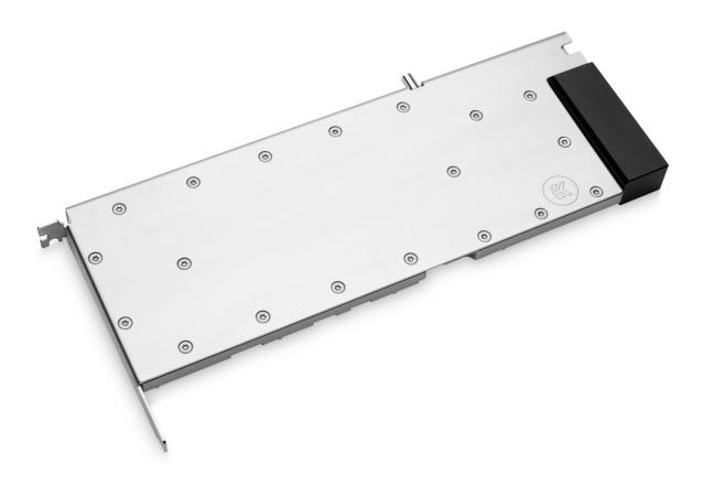
The base of the block is CNC machined out of nickel-plated electrolytic copper, while the top is laser-cut out of industry-grade stainless steel. The sealing is ensured by high-quality EPDM O-Rings. The brass standoffs are already pre-installed and allow for a safe and easy installation procedure.
