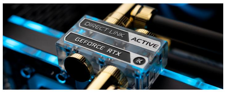
This terminal is CNC-machined out of glass-like cast acrylic.
