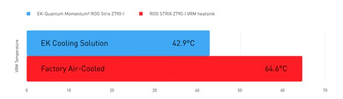
This monoblock uses the latest generation of EK-Quantum Velocity<sup>2</sup> cooling engine to ensure the best possible CPU cooling while not reducing flow to other components. The cooling engine uses a specific combination of mounting pressure and coldplate geometry tailored for the IHS and die layout of Intel LGA 1700 socket processors. It provides cooling for the heatsink of the voltage regulation module and 12th or 13th-Gen Intel Core™ CPU.
