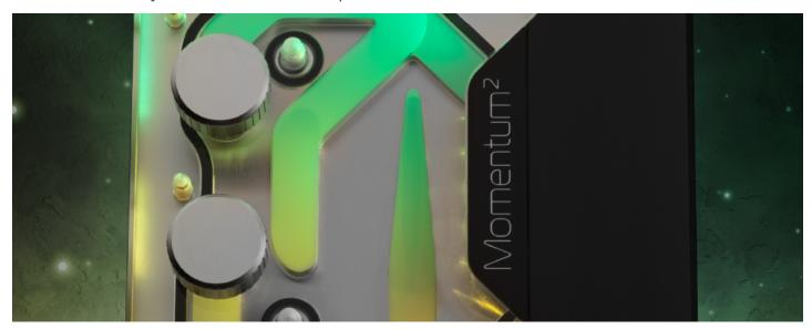
The base of the monoblock is made of nickel-plated electrolytic copper, while the top is made of quality cast acrylic material. The nickel-plated brass screw-in standoffs are pre-installed and allow for easy installation. Unlike other solutions on the market, this is a true one-piece, sturdy, and reliable liquid cooling product that requires only two connector fittings for proper operation. For the CPU, please use the enclosed (electrically non-conductive) thermal grease EK-TIM Ectotherm.
