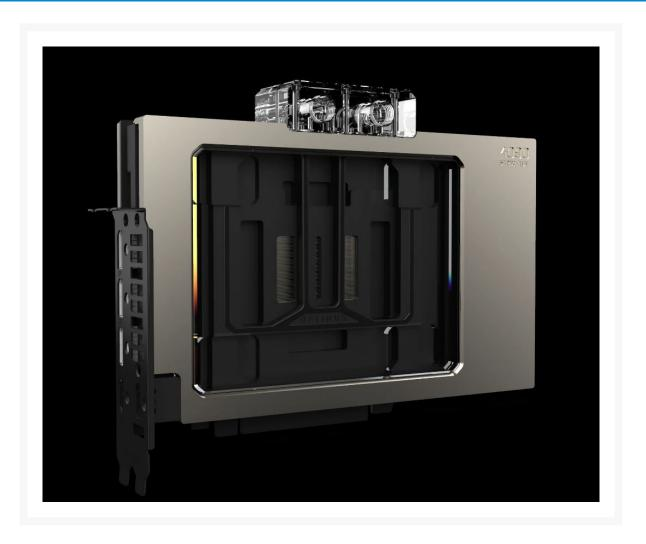
The new Signature Rev2 GPU block features increased performance and even higher mechanical reliability. The new cold plate plus improved brass midplate design reduces temps 1.5c over the previous design, thus increasing the potential overclocking by 15-30mhz. For reference, this puts the Signature block approximately 8-12c lower than competing blocks at the same wattage.
