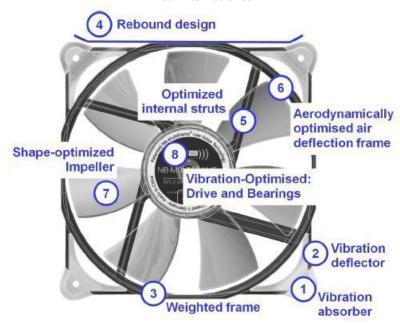
(1 + 2) Almost vibration-free construction through multipart frame design. The vibrations are passed through vibration deflectors to vibration absorbers. As a result the vibrations are almost completely eliminated in the frame of the fan. (3) A weighted frame provides additional vibration damping. Furthermore, the additional mass means that any opera
