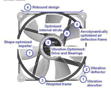
(1 + 2) Almost vibration-free construction through multipart frame design. The vibrations are passed through vibration deflectors to vibration absorbers. As a result the vibrations are almost completely eliminated in the frame of the fan.
