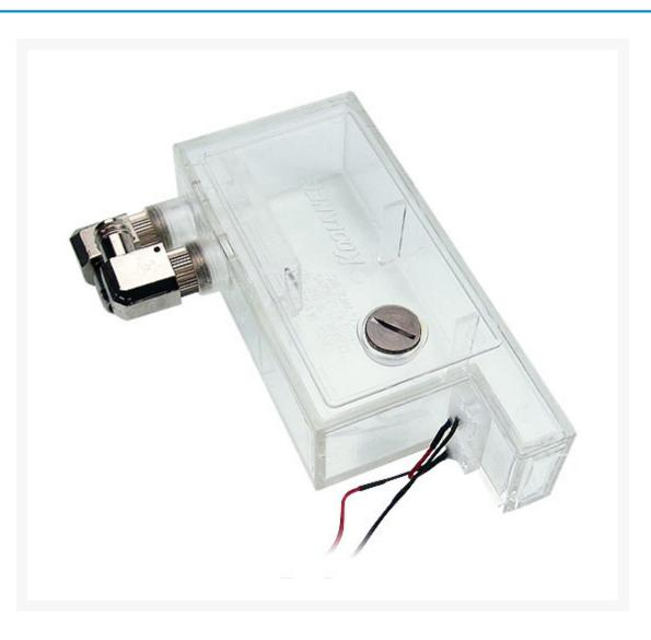
Reservoir used in the Koolance PC4-1000 series and RP-1000 products, usually combined with the PMP-400 pump. Includes blue LED tank lighting. Swiveling nozzles are 3/8" (10mm) ID, nickel-plated brass. Overall size including nozzles is 4.4" x 6.1" x 1.6" (11.2cm x 15.5cm x 4cm).
