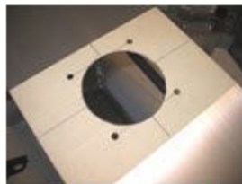
Cut a 4.5 hole for 120mm fan. 11/64 size drill bit for fan mounting holes.
