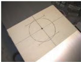
Use masking tape & ruler to measure location for 120mm cooling fan
