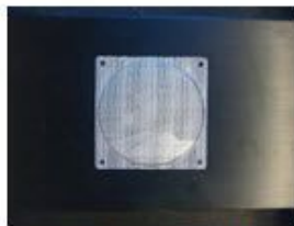
Place included grill over 120mm fan hole.
