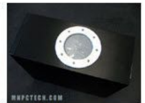
Installation Finished. 120mm Blowhole Kit
