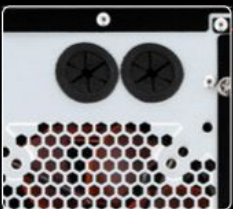
Pre-drill pipe holes for water cooling
