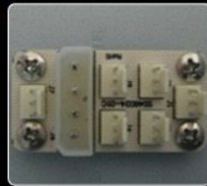
Added PCB provide extra fan Connection and reduce cable mess
