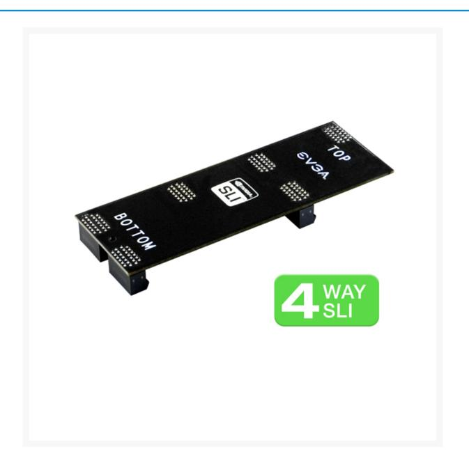
For use with 4-way SLI Capable Motherboards, Please note Top and Bottom designation as "TOP" must be placed on the top most (Primary) card to ensure proper 4-way SLI function.
