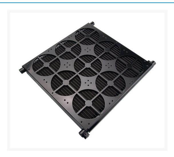
HX-1080 is the brazed aluminum heat exchanger used in the Koolance ERM-3K3UA cooling system, designed for 9 x 120mm fans. This version is enclosed in a steel frame with identical M4 threaded holes on both sides for mounting and fans. G 1/4" BSP inlet and outlet, 388x437x34mm, 2.8kg (6.2lbs). Enough BLT-HX025 hardware is included to mount all nine fans. NOTE: Hose barbs are recommended for this product to avoid conflict from one of the nozzle sockets.
