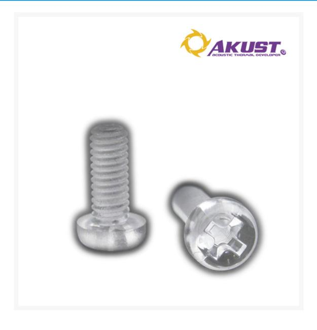
Akust Rustless machine screws are made out of Nylon 6/6. Which is a rust and corrosion resistant material that is also non-electrical conductive. It is lightweight and made of molded resin that is resistant to heat between 270-300 degrees F. Material has a tensile strength of 12,000 PSI.
