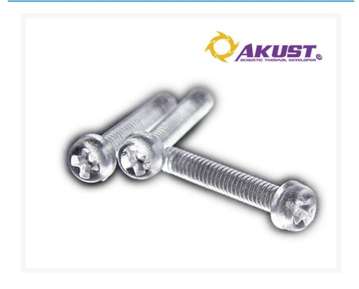
Akust Rustless machine screws are made out of Nylon 6/6. Which is a rust and corrosion resistant material that is also non-electrical conductive. It is lightweight and made of molded resin that is resistant to heat between 270-300 degrees F. Material has a tensile strength of 12,000 PSI.
