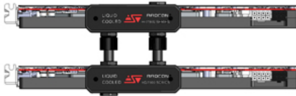
60mm/2.3" PCI spacing: Komodo HD7900 series waterblocks in CrossFireX with stock bridge
