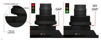
For complete long-term safety and leak-free operations, Swiftech® recommends that the fittings be locked in place using the recommended tools and that the torque levels specified below be applied:
