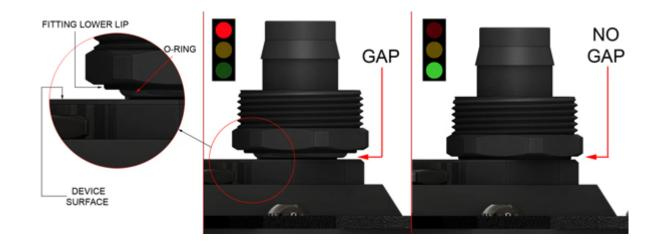
• For complete long-term safety and leak-free operations, Swiftech® recommends that the fittings be locked in place using the recommended tools and that the torque levels specified below be applied:
