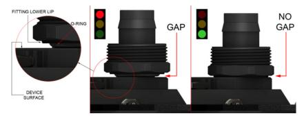
For complete long-term safety and leak-free operations, Swiftech® recommends that the fittings be locked in place using the recommended tools and that the torque levels specified below be applied:
