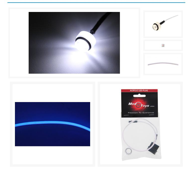
LED-lit plug from ModMyToys with G1/4" standard-screw thread and o-ring seal. The LED is powered directly from the power supply via the 4-pole connector plug). This LED-lighting set is compatible with all compensating reservoirs with 1/4" screw thread (i.e. Watercool AB-K, Eheim, etc).
